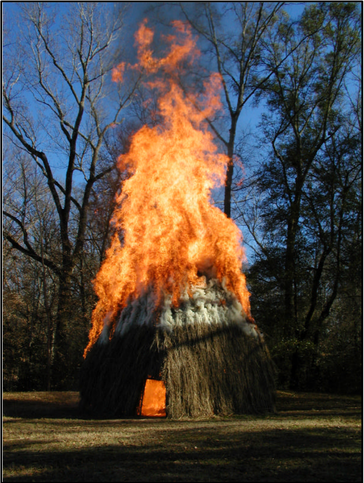
Figure 53. The experimental house after being set on fire from the inside, approximately 45 seconds after lighting the fire.
